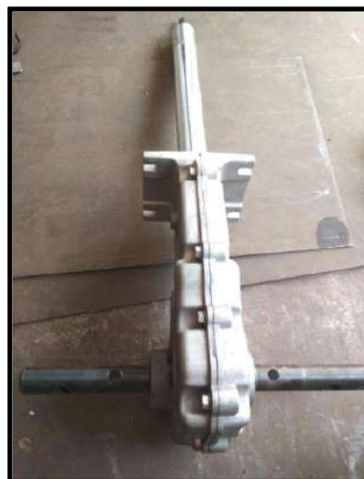
Fig. 2. Worm gear box fixed with rotor shaft
