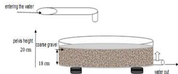
Fig. 1. Components of a vertical flow pretreatment basin
