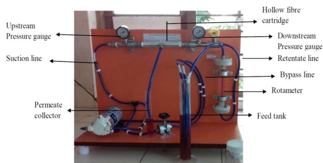
Plate 1. Hollow fibre membrane setup
