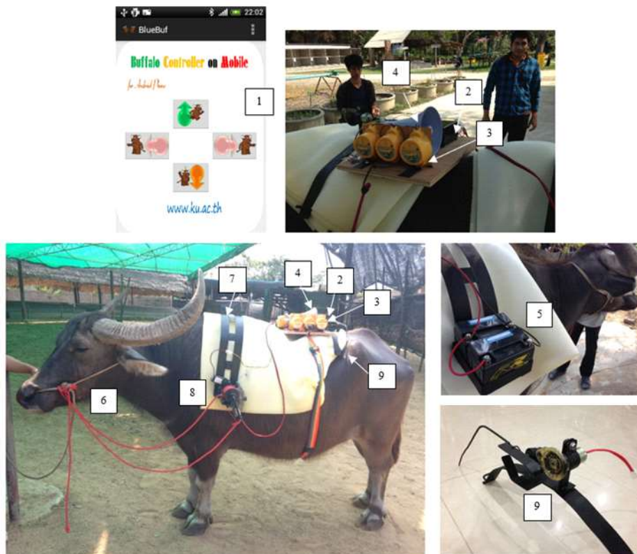
Fig. 2. Smartphone via bluetooth control device for commanding buffalos
