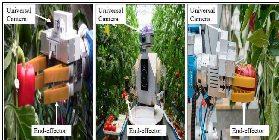
Fig. 7. Robotic harvesting with end-effector installed with universal camera
