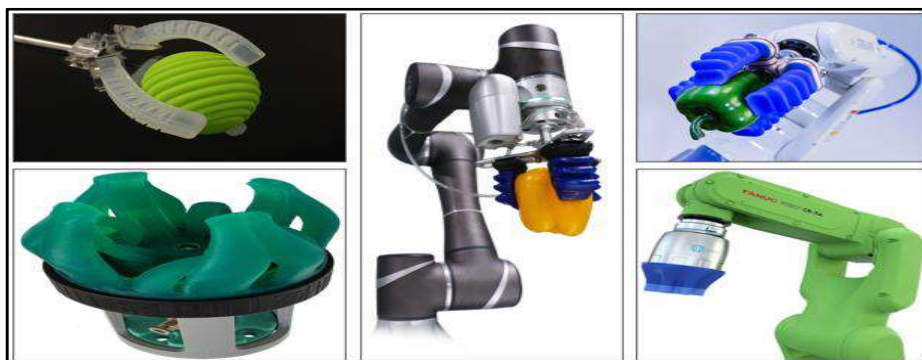
Fig. 8. Different types of soft and hollow fingers used in end-effector
