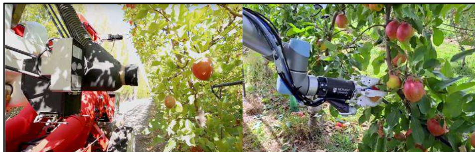
Fig. 4. Selective harvesting of apples with vision technology and end-effector manipulator
