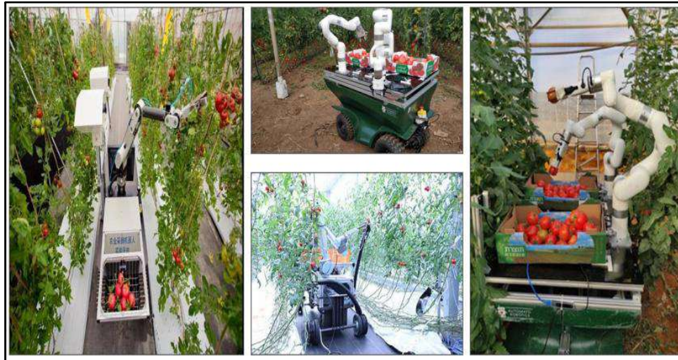
Fig. 12. Different types of robotic harvesters with autonomous collection and transportation mechanism
