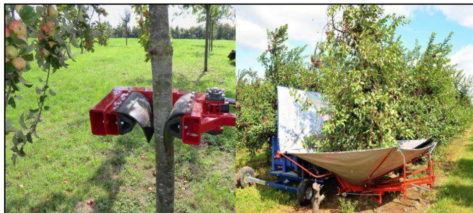
Fig. 6. Bulk harvesting method using mechanical tree shaker
