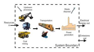
Fig. 6. Systems boundaries for a life cycle analysis of a coal fired power plant (Source: Spath, Mann, and Kerr, p. 4)
