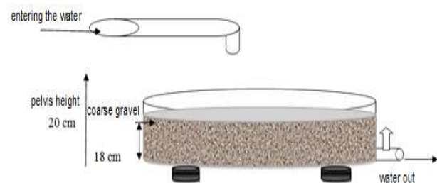
Fig. 1. Components of a vertical flow pretreatment basin
