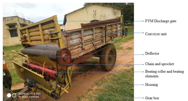
Fig. 8. Proto type tractor mounted FYM spreader fabricated under study
