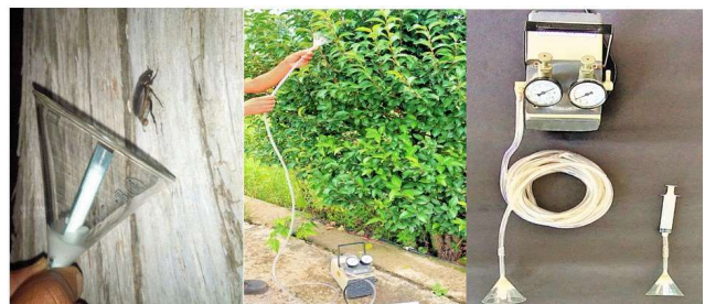
Fig. 1. Natural pheromone extracted through a handheld headspace sampling apparatus for in-situ volatile collection
