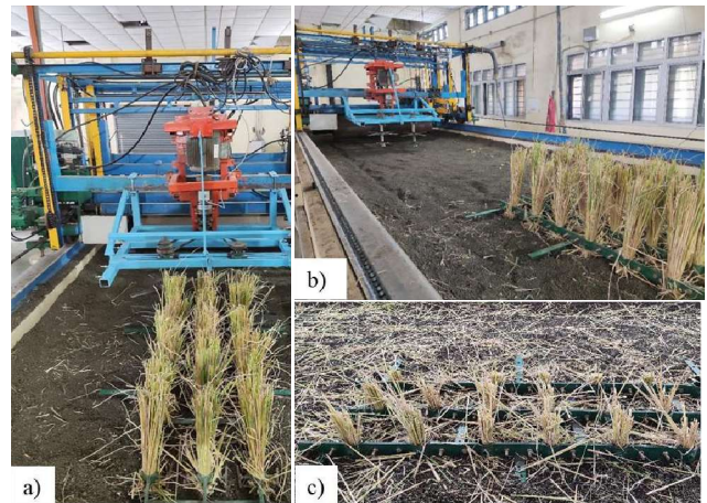
Fig. 2. a) Laboratory setup for cutting torque measurement, Paddy straw bunch in plant holder (b) before cutting and (c) after cutting
