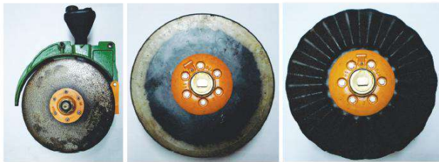
Fig. 5. Disc type furrow opener
