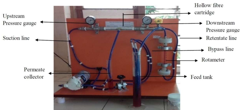
Plate 1. Hollow fibre membrane setup
