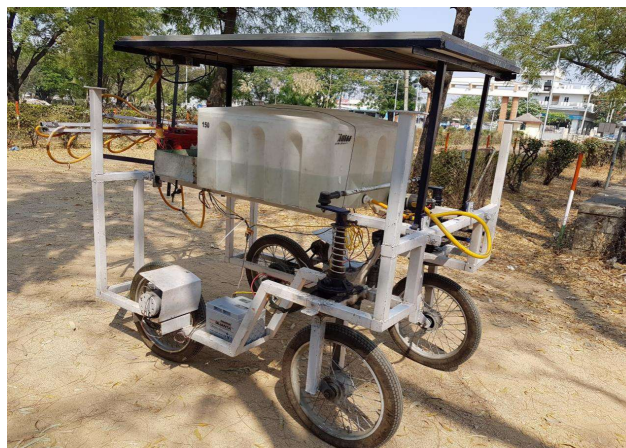
Fig. 2. Stationary view of solar powered remote-controlled sprayer
