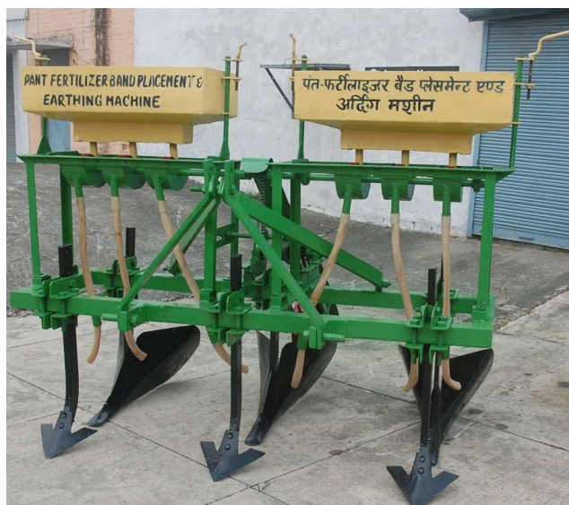
Fig. 1. Pant fertilizer band placement cum earthing machine
