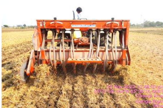
Use of Happy seeder for Zero tillage sowing of wheat in Paddy harvested field
